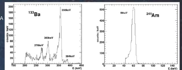
An energy resolution of 9.2keV (FWHM) at 356keV (<sup>133</sup>Ba source) and 5.47keV (FWHM) at 59.5keV (<sup>241</sup>Am source) for one pixel
