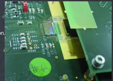
CdTe pixel detector in a stack configuration
