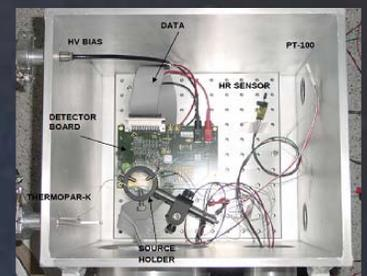
Experimental set-up inside the vacuum chamber
