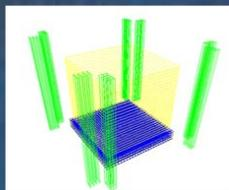
Model mass of a Si/CdTe Compton Camera
