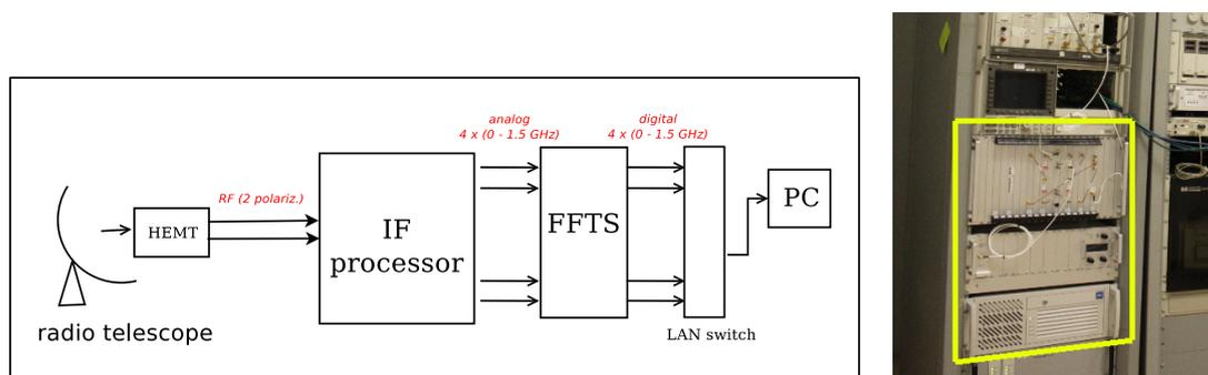
Figure 3: *Left panel:* A concept diagram of the wideband backend. *Right panel:* The backend installed. It is possible to see the IF processor, the FFT spectrometer and the PC which controls the observations.
