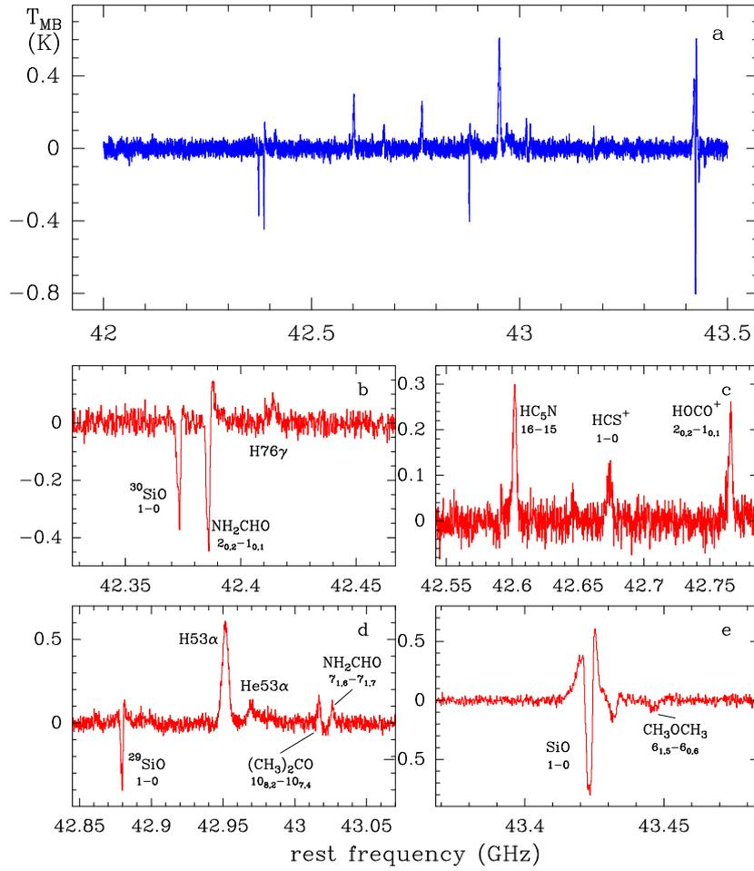
Figure 5: A spectrum of Sgr B2(M) at Q-band, obtained with the new wideband backend and the new receiver, attached to the DSS-54 antenna. This spectrum, of 1.5 GHz of bandwidth, was obtained after only 20 minutes of integration time.
