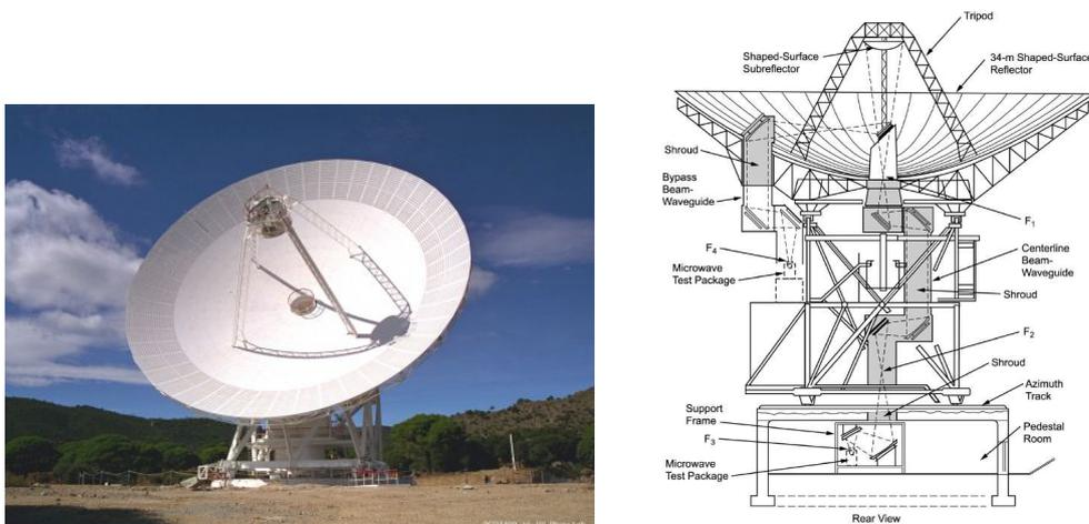
Figure 1: *Left panel:* Photograph of the DSS-54 antenna. *Right panel:* A beam waveguide schematic. (Credit: JPL)
