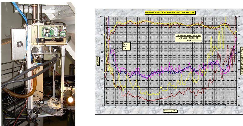
Figure 2: *Left panel:* Photograph of the  $Q$ -band receiver. *Right panel:* Chart of the receiver temperature and Y-factor. (Credit: JPL)
