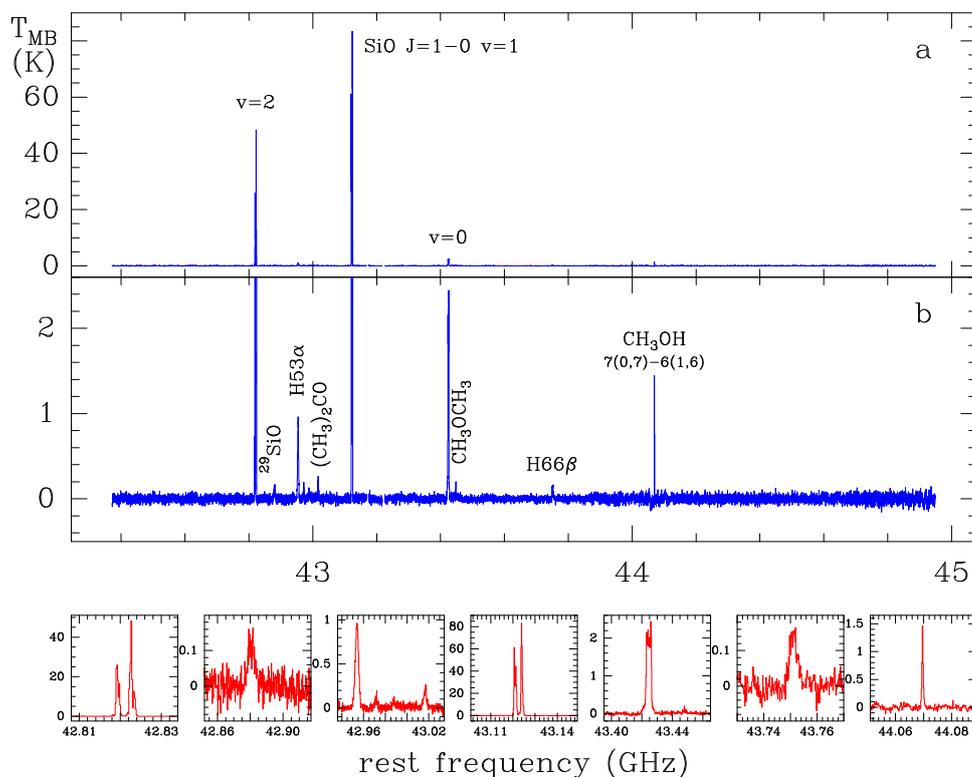
Figure 4: A spectrum of Orion KL at Q-band, obtained with the new wideband backend and the new receiver, attached to the DSS-54 antenna. Bandwidth is 2.6 GHz.
