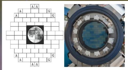
Figure 1: Left Panel, Schema of the DECam focal plane Right Panel, real camera.
