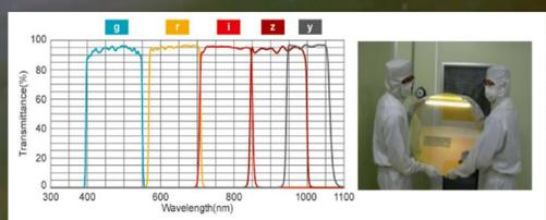
Figure 2: Filter system will be used on DES according to the wavelength. Right, one of these filters.
