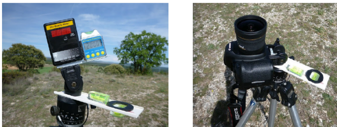
Figure 2: Left panel: SQM-L photometer mounted on tripod and pointing 20 degrees from zenith. Right panel: DSLR camera and fish eye lens providing all-sky view of the sky.
